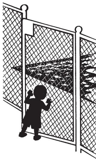
When the release mechanism of the self-latching device is less than 54 inches from the bottom of the gate, the release mechanism for the gate should be at least 3 inches below the top of the gate on the side facing the pool. Placing the release mechanism at this height prevents a young child from reaching over the top of a gate and releasing the latch.
