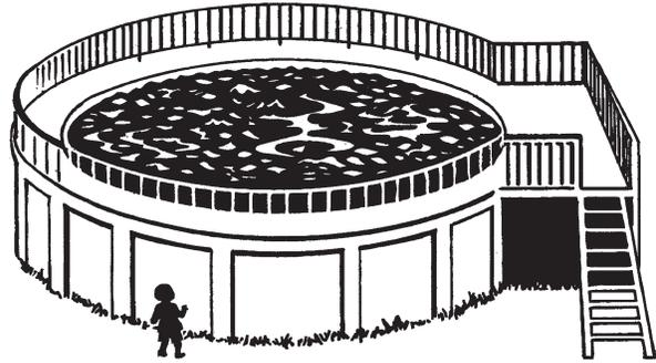
Aboveground pools should have barriers. The pool structure itself serves as a barrier or a barrier is mounted on top of the pool structure.
