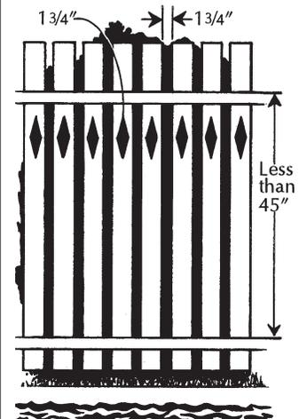
If the distance between the tops of the horizontal members is **more** than 45 inches, the horizontal members can be on the side of the fence facing away from the pool. The spacing between vertical members should not exceed 4 inches. This size is based on the head breadth and chest depth of a young child and is intended to prevent a child from passing through an opening. Again, if there are any decorative cutouts in the fence, the space within the cutouts should not exceed 1-3/4 inches.
