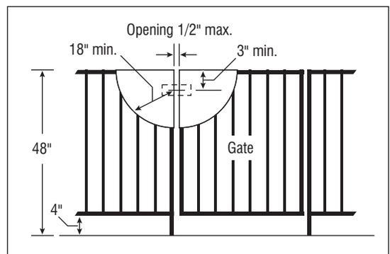
**Use this as a guide when the release mechanism is located less than 54 inches from the bottom of the gate.**
